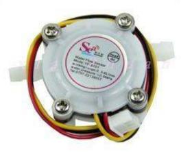
Water flow sensor consists of a PVC body, a water rotor, and a hall-effect sensor. When water flows through the rotor, rotor rolls. Its speed changes with different rate of flow. The hall-effect sensor outputs the corresponding pulse signal. This one is suitable to detect flow in water dispenser or coffee machine.
