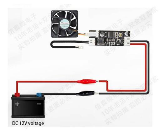
$\Box$  . This controller is designed as a model that combines manual control and automatic temperature control.
