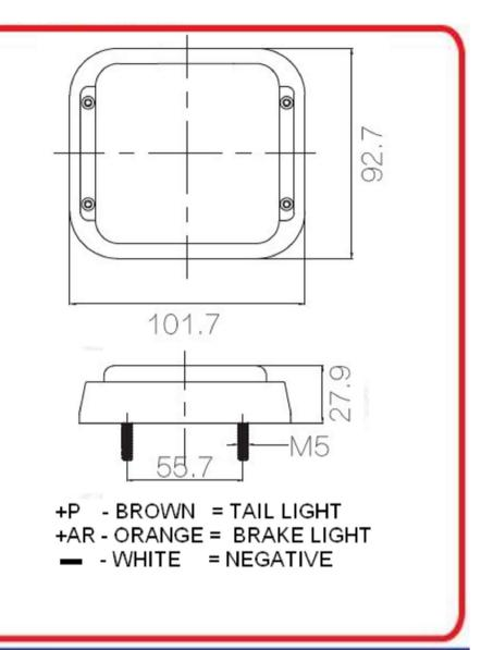
Stop and Rear Position Lamps/ FLASHING LAMP
