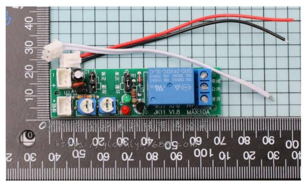
This module adopts single chip microcomputer as the main control core, with high time precision. SCM has built-in watchdog circuit and reset chip, which works stably and reliably.
