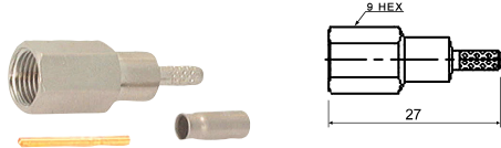
M577502 FME male crimp type gold-pin (RG58U/174U)
