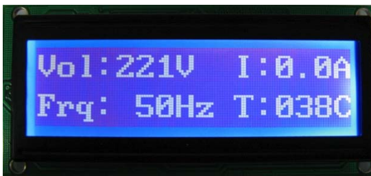
Figure 8.8c: Display on LCD when EG8010 connects to 12832
