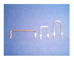
These simple, yet robust designs exhibit extremely low resistance (3 milliohms), which is suitable for high power current detection. Dimensions and pitch are both variable. These models are easy to solder. They are also non-inductive.
