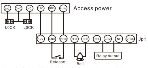
**Remark:** If let relay drive electric-lock, please connect a reverse diode with the lock's "+" and "-" poles.
