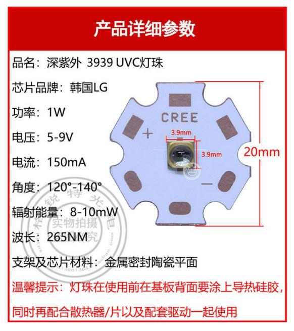
Product Parameter Product Name: 3939UVC Lamp bead Chip Brand: KOERA LG Power: 1W Voltage: 5-9V Current: 150mA Degree: 120° -140° Radiant Flux: 8-10mW Peak Wavelength: 265NM Bracket and chip materials: Metal seal and Ceramic flat Warm tips: The lamp bead should be coated with heat-conducting silica gel on the back of the substrate before use, and used together with the radiator and matching drive at the same time.
