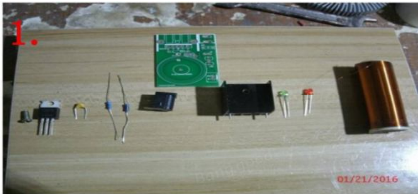
PCB board x 1, monolithic capacitors x 1, 10K, 1K resistor each x 1, LED x 2, 12V power socket x 1, heat sink x 1, transistor x 1, secondary coil x 1, fixing screw x 1. Resistance, left the right side of 1K 10K
