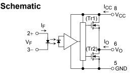
A 0.1  $\mu F$  bypass capacitor must be connected between pins 8 and 5. (See Note 6)
