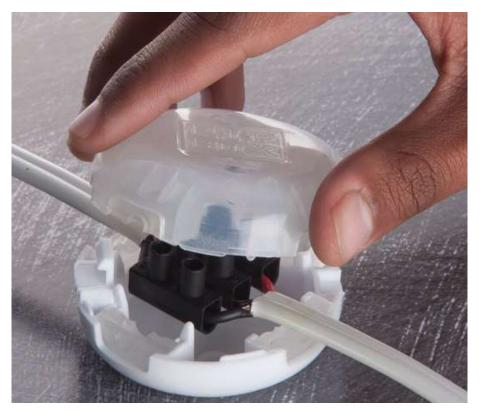
Two identical halves clip together over a new or existing electrical wire connection to form a compliant junction box, without having to disconnect and reconnect the wires.
