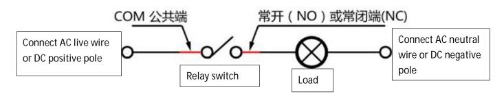
When the relay switch closes, and plant has voltage on both side of end, the relay can normally work. When the relay switch is disconnected and it can't work.
