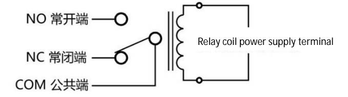
When there is no voltage or voltage is not enough on both ends of relay coil, COM and NC of relay will be connected.
