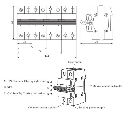
Switch wiring diagram
