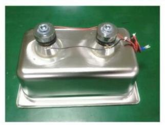
After the glued and solidified for 24h, it can be connected to oscillator wire, distinguish the positive and negative poles. The red wire is the positive and the black wire is the negative pole, which cannot be connected reverse.
