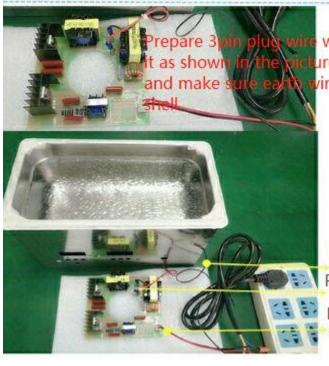
with earth wire, and connect ture. Can't connected reverse, wire connected the metal
