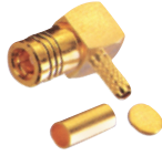
M5151 SMB FEMALE CRIMP TYPE (RG174U/178U) (GOLD PLATED)
