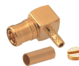
M516005 RIGHT ANGLE SMB FEMALE CRIMP TYPE (RG174U/178U) (GOLD PLATED)
