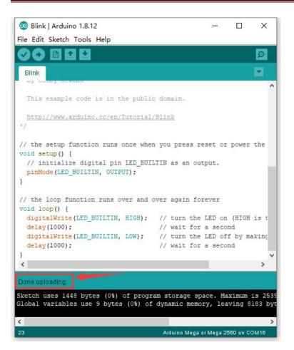
After the program is uploaded successfully, the onboard LED blinks.
