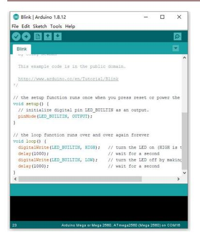
Set the correct **COM port**, and the corresponding board and COM port are shown on the lower right of IDE.
