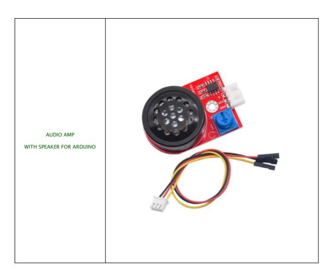
The keyestudio power amplifier module integrates an adjustable potentiometer, a speaker, and an audio amplifier chip.
