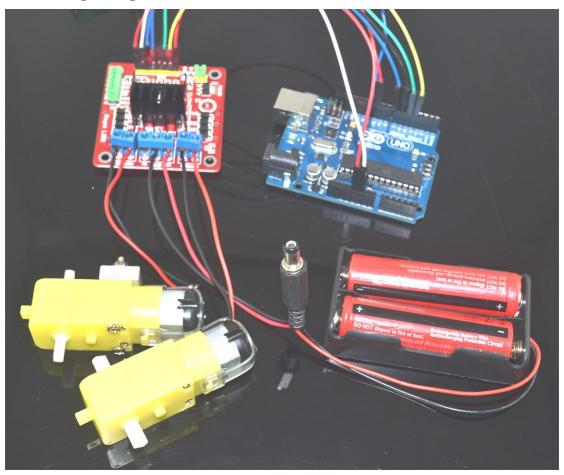
Note: The digital ports 4 and 5 are one set, and 6 and 7 are another set. Digital ports 10 and 11 are used as the enable ports of the DC motor.
