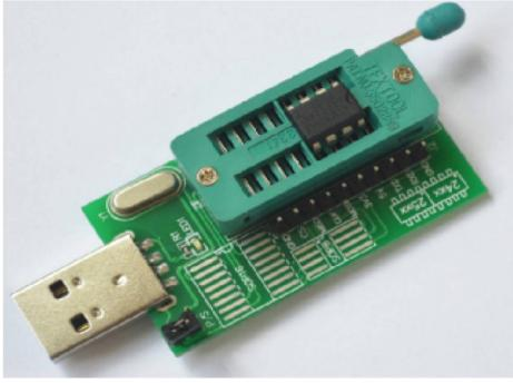
2: Insert the programmer into the USB port of the computer and open "CH341A programmer 1.17" Programming software in. Select the chip, you can program and erase the chip.
