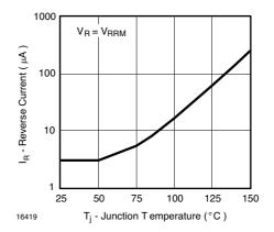
Figure 4. Reverse Current vs. Junction Temperature
