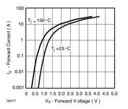
Figure 2. Forward Current vs. Forward Voltage
