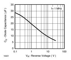
Figure 6. Diode Capacitance vs. Reverse Voltage
