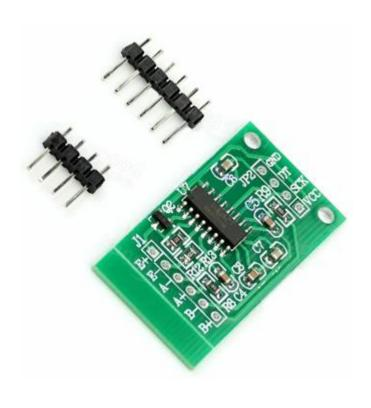
The module uses 24 high-precision A/D converter chip HX711. It is designed specifically for high-precision electronic scales. With two analogue channel inputs and programmable amplifier gain. The input circuit can be configured for electrical bridge (bridge pressure as the pressure weighing) sensor mode is ideal for high-precision, low-cost sampling front-end module.
