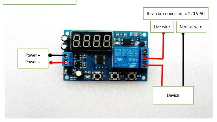
Working mode selection: after power on, press and hold K1 for 2 seconds to enter the selection function mode, P1-1 ~ P1-3 can be selected;
