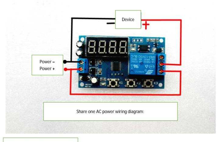
Control 220 V circuit wiring diagram
