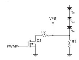
$$MOSFET 'off' \\ I_{LED(MIN)} = \frac{V_{FB}}{R_{LED}}$$
