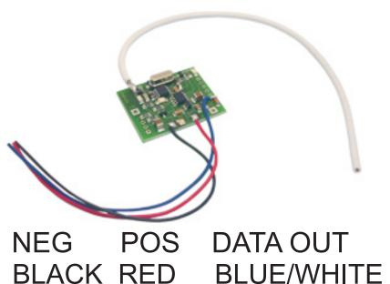
Connect 5v DC to transmitter and receiver Data sent into transmitter will be received out at receiver, single direction communication
