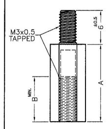
NOTE:(1)Inner thread was done by 2nd process taping.
