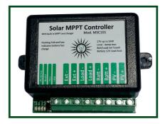
A microprocessor controls the MPPT operation and simultaneously charges and maintains the battery from a solar panel, and controls a load, with day/night switch capability. When the battery drops to 11.0V, the unit switches the load to the external supply, ensuring your load is always powered when required even when the battery is flat.
