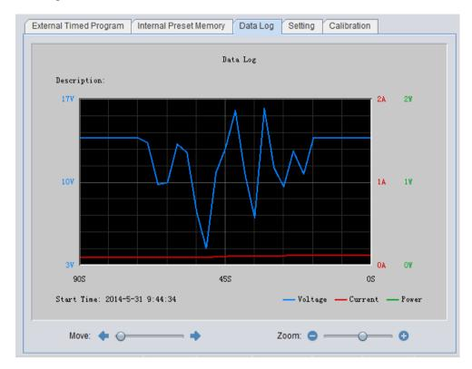
Data log window is used to display output Voltage, Current and Power against time in graphical view. You can move the diagram left and right by adjust "Move:" slide bar.
