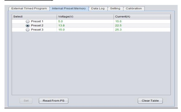
The PC interface remote mode really eliminates the tedious process in keying in groups of entries on the power supply. Because all the data are displayed together in the monitor, possibility of wrong entry is greatly reduced. Data of different groups can be classified, stored, exported and retrieved for use at any time.
