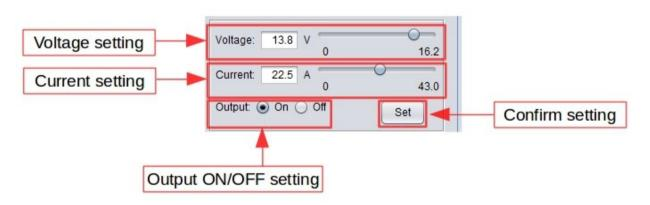
You can directly type the desired output voltage & output current and then click "Set" button to set the value. Or you can use slide bar to adjust the value.
