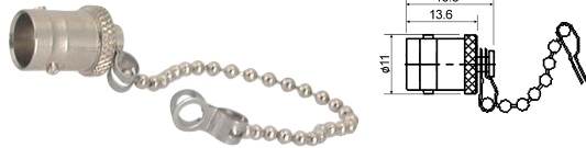
M55783 BNC male terminator gold-pin A: 50 Ω B: 75 Ω C: 93 Ω
