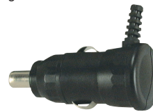
K32087 Auto plug to USB/A adapter W/fuse/2A W/short circuit / over voltage / reverse protection W/LED In:12V/24V Out:5V 0.5A
