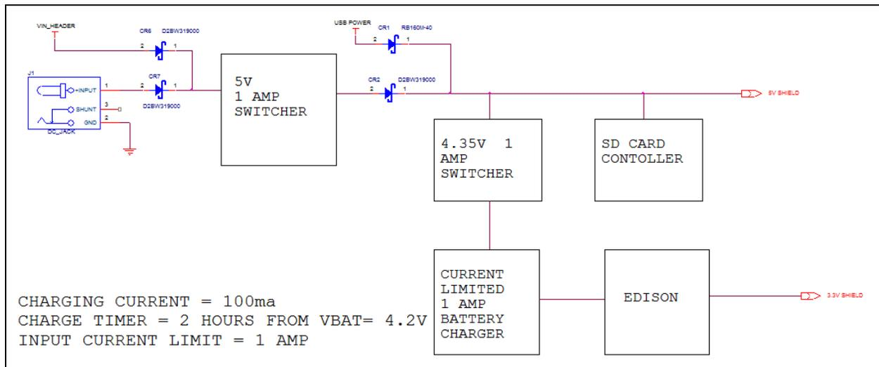
Power from the 5 V switcher is diode-ORed with power from the USB connector. This arrangement allows the Intel® Edison kit for Arduino\* to run off external power or USB power. This rail is used to power the shields, the SD card slot, and a 4.35 V switcher. The total current on this rail should be limited to 1 A maximum continuous.
