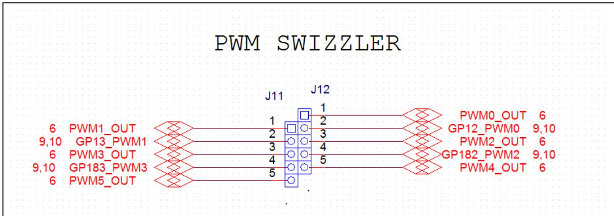
The four PWM sources from the Intel® Edison board GP12\_PWM0, GP13\_PWM1, GP182\_PWM2, and GP183\_PWM3 can be configured to drive four of the six Arduino header PWMs. Each Intel® Edison board PWM can be jumpered to one of three Arduino PWMs. For example, GP12\_PWM0 can be jumpered to PWM0\_OUT, PWM2\_OUT, or PWM1\_OUT.
