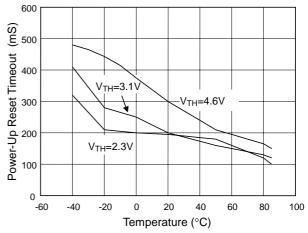
Fig 6 Power-Up Reset Timeout vs. Temperature
