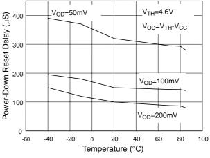
Fig 4 Power-Down Reset Delay vs. Temperature
