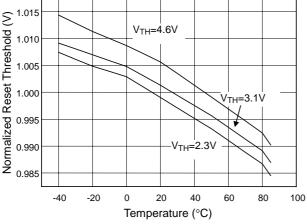
Fig 5 Normalized Reset Threshold vs. Temperature
