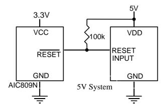
Fig. 8 Open-Drain Output Allows Use with Multiple Supplies
