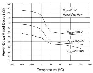
Fig 2 Power-Down Reset Delay vs. Temperature
