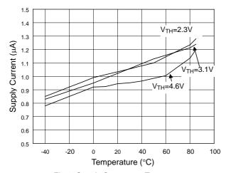
Fig 1 Supply Current vs. Temperature
