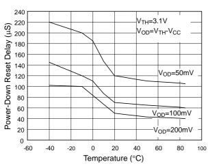
Fig 3 Power-Down Reset Delay vs. Temperature
