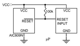
Fig. 7 Open-Drain Output
